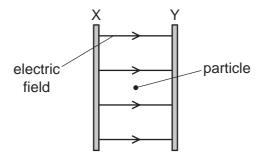
The particle moves towards plate X when the p.d. is applied.
