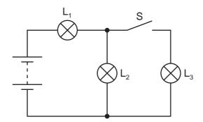
What happens to the brightness of lamps L<sub>1</sub> and L<sub>2</sub> when the switch S is closed?
